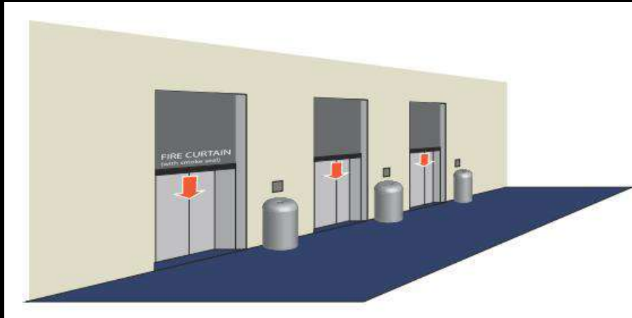
LIFT LOBBY & ELEVATOR SEPARATION
